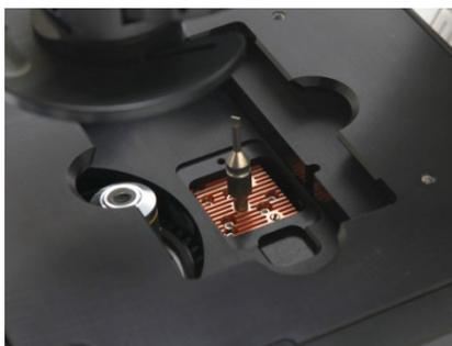
6. Use the tool to tilt the light cube slightly toward you and lift out gently, and then remove tool from cube.
